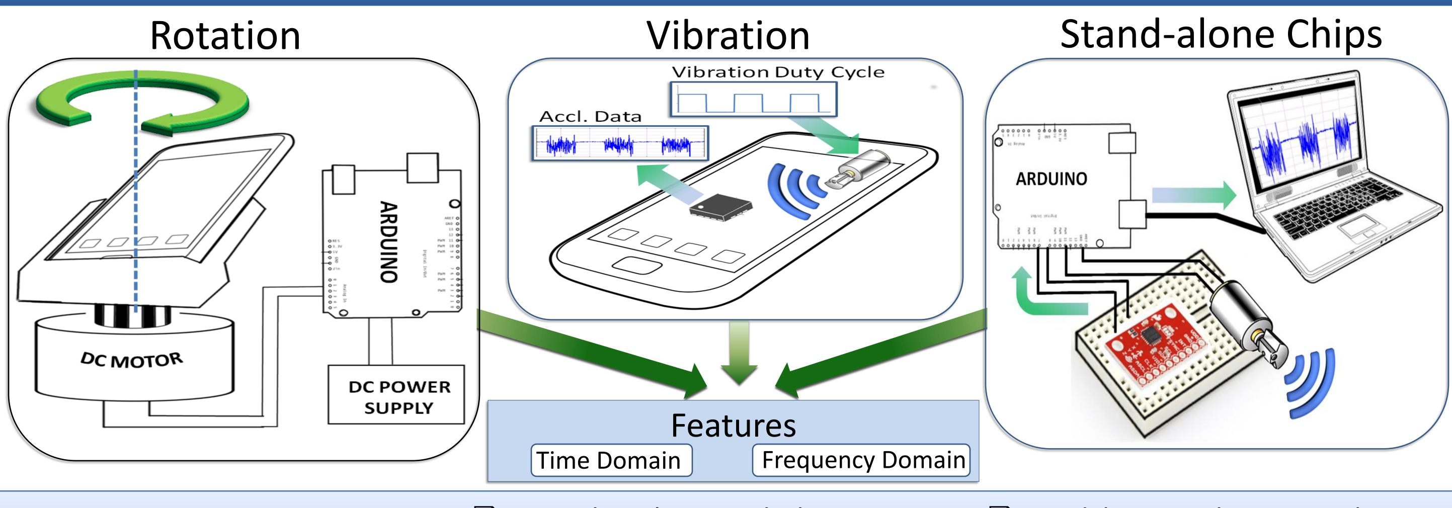
DC motor is used to generate fixed pattern of stimulation
