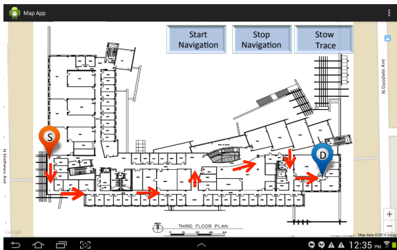
Figure 2: Allocentric interface with the marker for source, destination and traveled track on the schematic map.
