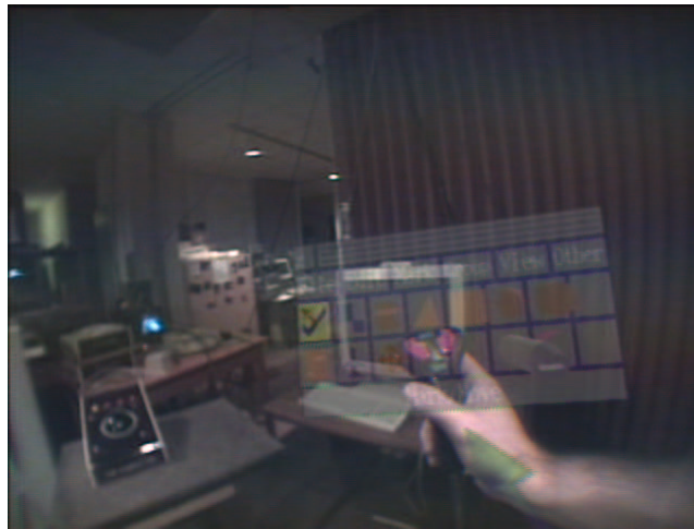
Figure 1a - a simulation of an optical see-through HMD
