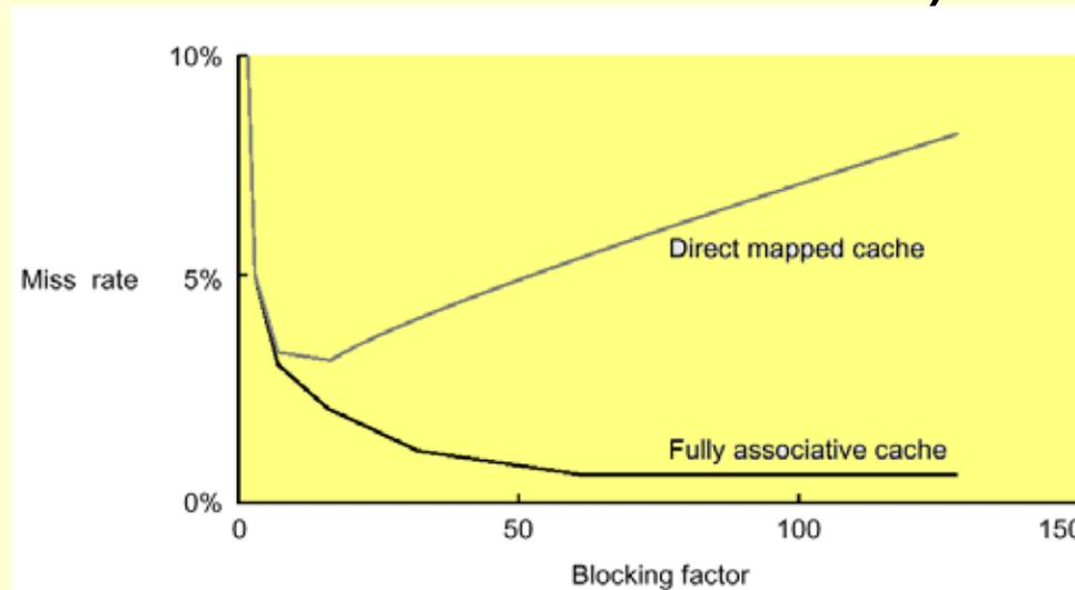
Lam et al [1991] a blocking factor of 24 had a fifth the misses compared to a factor of 48 despite both fit in cache
