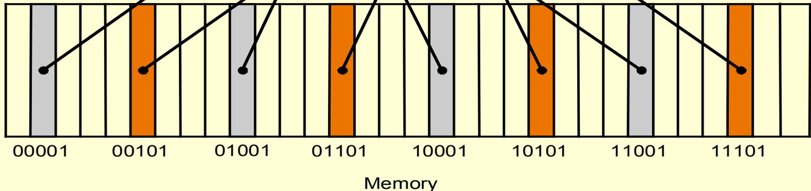
$$\text{Cache block address} = (\text{Block address}) \bmod (\text{Number of cache blocks})$$
