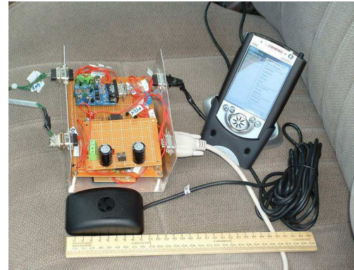
Figure 2: VEDAS system connected to a car. The scantool is connected to the car through the OBD-II connector. A GPS device is connected for location information and the iPAQ downloads the data from the car for analysis.
