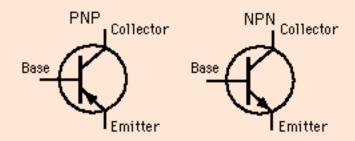
A bipolar junction transistor consists of three regions of doped semiconductors. A small current in the center or base region can be used to control a larger current flowing between the end regions (emitter and collector). The device can be characterized as a current amplifier, having many applications for amplification and switching.
