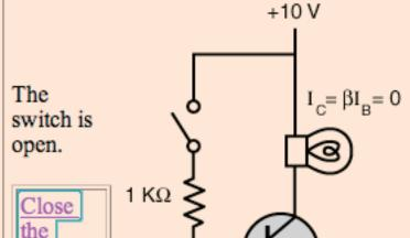
There is no current to the base. so the transistor is in the cut off condition with no collector current. All the voltage drop is accoss the transistor.
