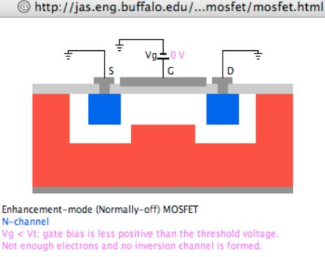
N-channel Vg < Vt: gate bias is less positive than the threshold voltage. Not enough electrons and no inversion channel is formed.
