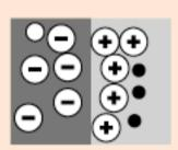
Filling a hole makes a negative ion and leaves behind a positive ion on the n-side. A space charge builds up, creating a <u>depletion region</u> which inhibits any further electron transfer unless it is helped by putting a <u>forward bias</u> on the junction.
