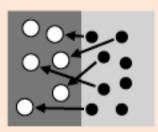
When a <u>p-n junction</u> is formed, some of the electrons from the n-region which have reached the <u>conduction band</u> are free to diffuse across the junction and combine with holes.
