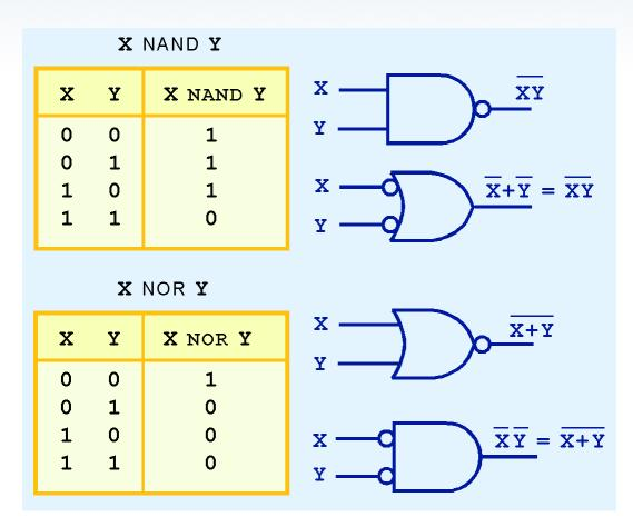
NAND and NOR are known as universal gates because they are inexpensive to manufacture and any Boolean function can be constructed using only NAND or only NOR gates.
