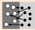
When a p-n junction is formed, some of the electrons from the n-region which have reached the conduction band are free to diffuse across the junction and combine with holes.
