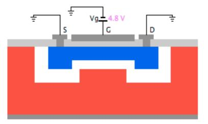
Enhancement-mode (Normally-off) MOSFET N-channel Vg > Vt: gate bias is more positive than the threshold voltage. Sufficient electrons accumulate and forms the inversion channel.
