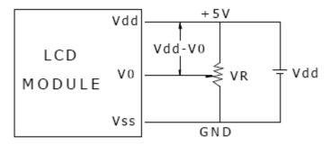
Vdd-V0: LCD Driving Voltage
