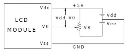
Vdd-V0: LCD Driving Voltage
