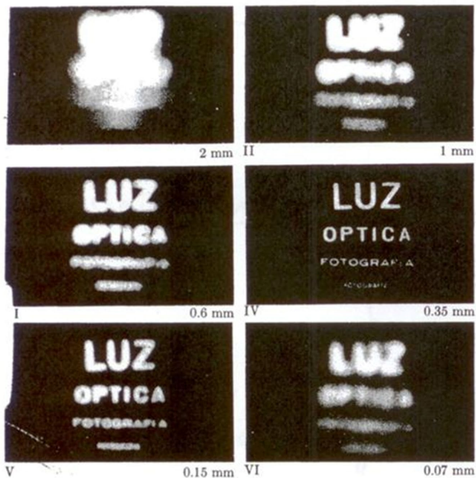
Fig. 5.96 The pinhole camera. Note the variation in image clarity as the hole diameter decreases. [Photos courtesy Dr. N. Joel, UNESCO.]
