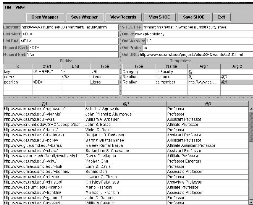
Figure 2. Running SHOE. A user can specify delimiters for recognizing fields and records, verify that they are extracted correctly, then create templates that translate the data into SHOE format.
