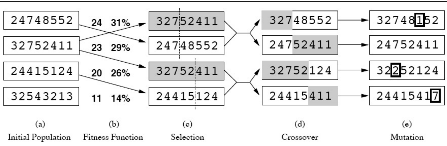
Figure 4.6 The genetic algorithm, illustrated for digit strings representing 8-queens states. The initial population in (a) is ranked by the fitness function in (b), resulting in pairs for mating in (c). They produce offspring in (d), which are subject to mutation in (e).
